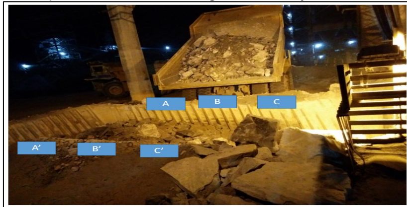
Fig. 5 Different Points at the Edge of Hopper at which Illuminance Level was Measured
