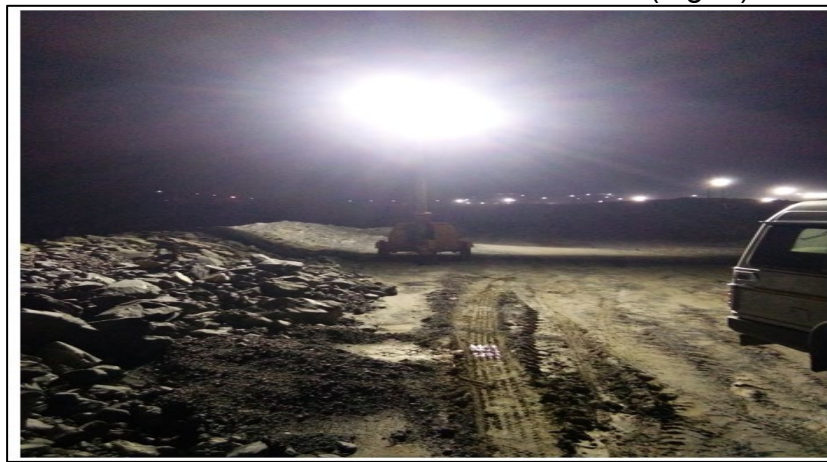
Fig. 2 Portable DG Tower at Intersection of Haul Roads in Quarry-2, 6 of Mine1
