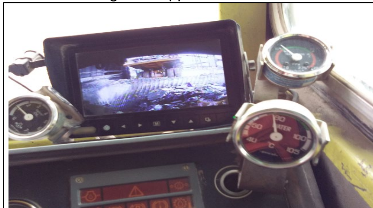
Fig. 6 Rear Vision Camera Showing View of Hopper Chute
